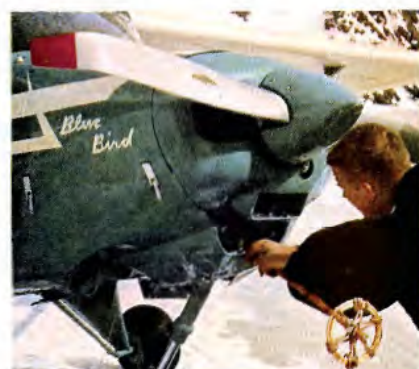
USING A SKI POLE as lever, Neal straightens damaged tubing. Blues spent half day welding wheel and bending prop into shape. Next try was successful and Blue Bird flew over Chilean Andes to Argentina and Buenos Aires.
