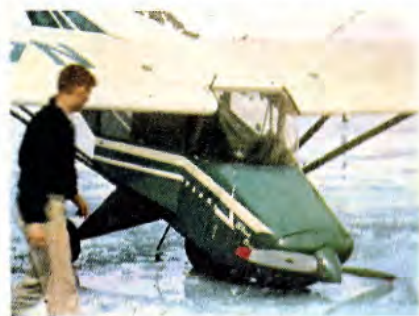
A DAMAGED NOSE WHEEL , buckled in take-off try is examined by Neal. Before starting their final run the boys tested the surface of the ice, but on take-off the nose wheel dropped into a two-foot fault and collapsed.
